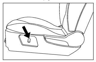
The power lift seat switch is located on the outboard side of the driver's seat. To raise or lower the seat, press the top or bottom of the switch.
